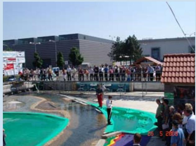
The picture shows the river flow model. It consisted of the river bed, a polder, a floodplain forest, settled area with colour-coded degrees of flood activity, a fish pass, a weir and a lock. A fully operational limnigraph station was set up in the exhibition to measure flow rates and water level heights in the channel, and the readouts were shown online on a large LED screen.
